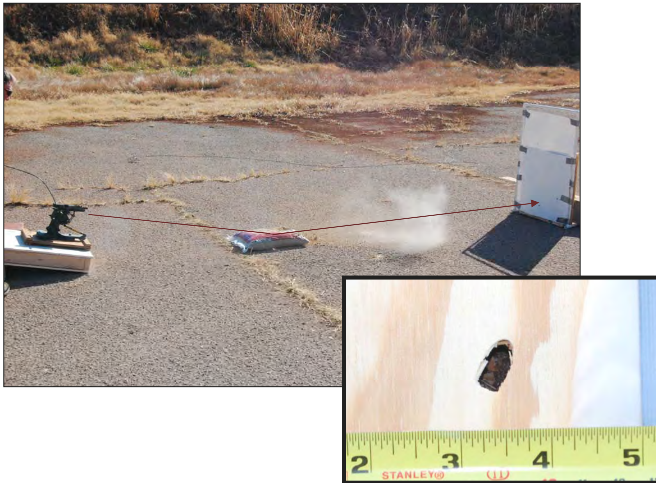
Figure 6- An impact site from a fired bullet that struck an intermediate object (the sand) first (the bullet originated from essentially 90 degrees-straight ahead). The intermediate object caused the bullet to tumble and enter the panel sideways and with the nose upward.
