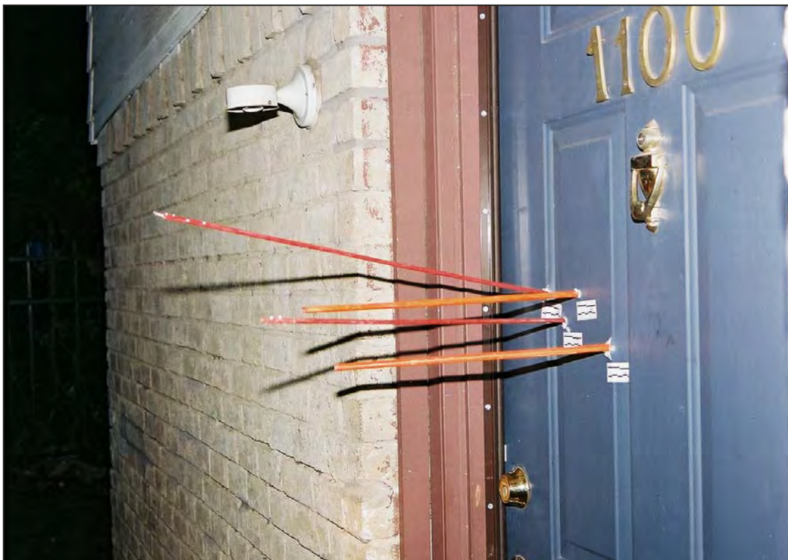
Figure 2-Original scene image of the exit side of the door through which shooter "A" delivered 4 shots-only three of these can hit the opposite wall.
